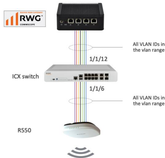
FIGURE 13 – VLANs WITH TAGGED INTERFACES IN THE ICX SWITCH
